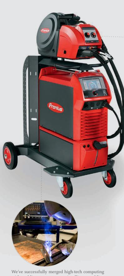
We've successfully merged high-tech computing with welding to create our intelligent welding system. This power source utilizes high speed communications to adapt the arc to minute changes during application.
