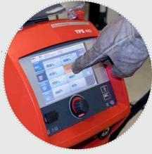
Touch screen controls make many aspects of welding easier. From learning to use the system to making parameter changes on the fly, everything can be accomplished without removing your gloves.
