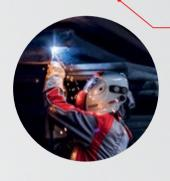
This helmet provides excellent protection which auto-darkens in as little as 0.05 seconds! With a default darkness level of 2.5, it makes seeing the workpiece prior to igniting the arc easy.
