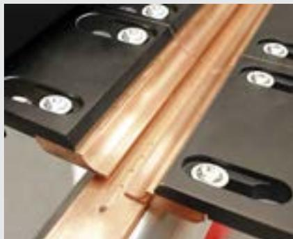
/ Backing track with forming gas holes
