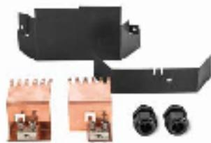
The DC Con Kit enables the connection of both inputs in the event of MPP currents above 35 A and a cable cross section of more than 16 mm<sup>2</sup>, for example when using a DC Box. The DC Con Kit 35 allows for cross sections of up to 35 mm<sup>2</sup>, which means that a maximum distance between inverters and modules can be covered. The terminal is safe to touch. The DC connector kit is particularly suitable for use with the Fronius Symo 10.0 - 20.0 kW and Fronius Eco inverters.
